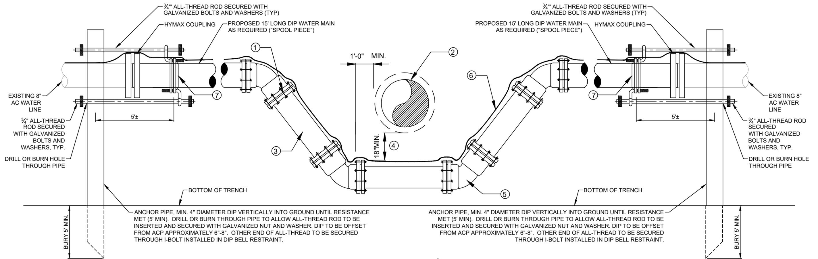
ANCHOR PIPE, MIN. 4" DIAMETER DIP VERTICALLY INTO GROUND UNTIL RESISTANCE MET (5' MIN). DRILL OR BURN THROUGH PIPE TO ALLOW ALL-THREAD ROD TO BE INSERTED AND SECURED WITH GALVANIZED NUT AND WASHER. DIP TO BE OFFSET FROM ACP APPROXIMATELY 6"-8". OTHER END OF ALL-THREAD TO BE SECURED THROUGH I-BOLT INSTALLED IN DIP BELL RESTRAINT.
