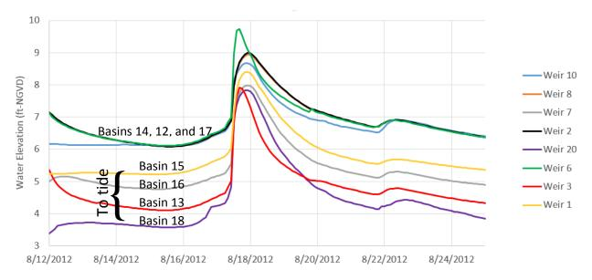
Figure 29. Hydrographs for the Lower Basins of Cape Coral for the first 13 days of the 25yr Design Storm simulation with Existing Conditions.
