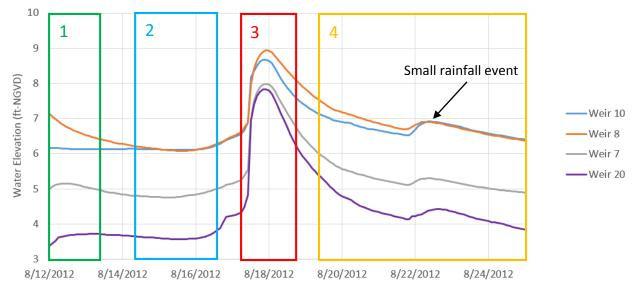
Figure 30. Depiction of the different phases of Basin drainage during a 25 yr Design Storm
