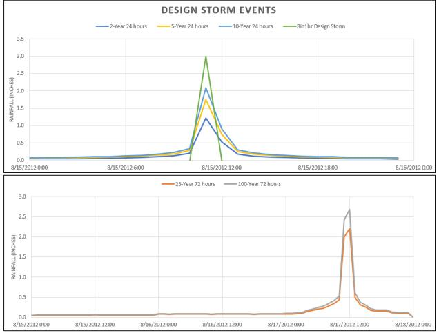
Figure 16. The rainfall intensity curves for the developed into the Design Storm simulations. The short duration events are shown on the top and the long-duration events are shown on the bottom.
