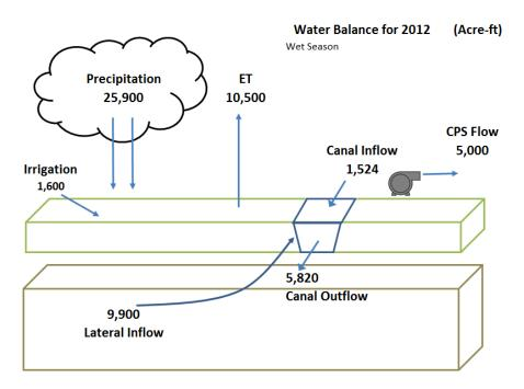
Figure 13 Water Balance schematic for the Southern Basins in acre-ft.
