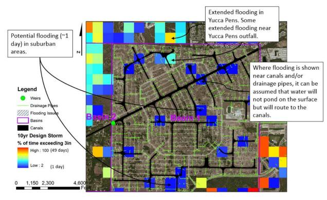
Figure 20. Secondary flooding in Basin 1. The colored squares indicate the percent of time that there is more than 3 inches of water during the 10 year Design Storm simulation.
