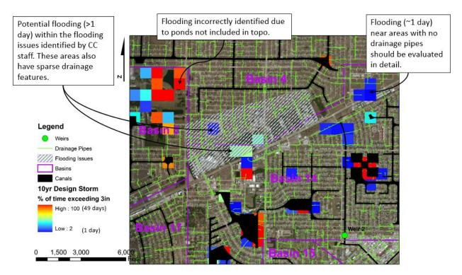
Figure 22. Secondary flooding in Basin 4 and 14. The colored squares indicate the percent of time that there is more than 3 inches of water during the 10 year Design Storm simulation.
