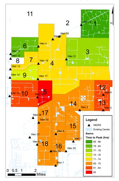
Figure 31. Map of the time to peak water elevation for critical Basins in the City of Cape Coral with existing structures and operations.
