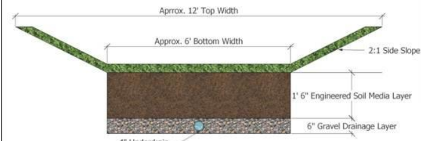
Example Vegetated Swale Cross Section
