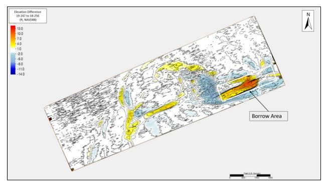
Figure 21: Borrow Area Post-Construction to Year 1 Monitoring Bathmetry Change
