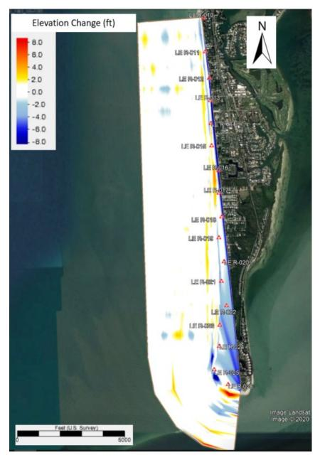
Figure 16: Elevation Changes between Post-Construction and Year 1 Monitoring Surveys
