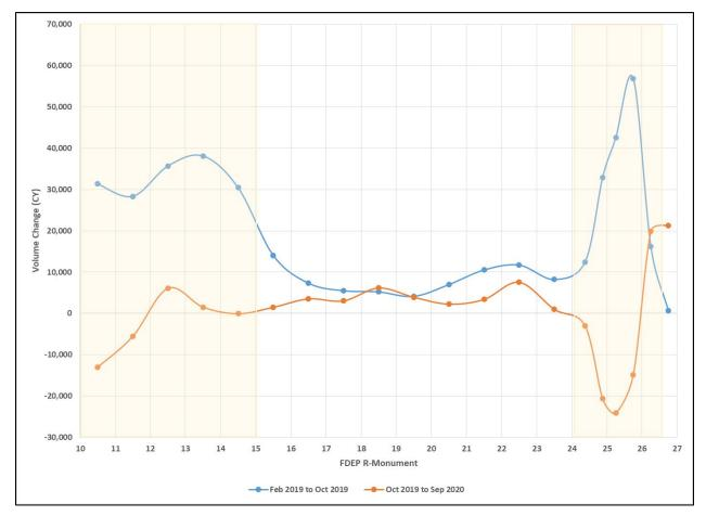
Figure 14: Volumetric Change from Dune To -13 Ft NAVD88 in the Beach Fill Area
