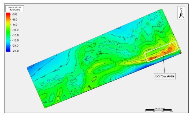
Figure 17: Pre-Construction Borrow Area Depths (Survey 18-256, December 2018)
