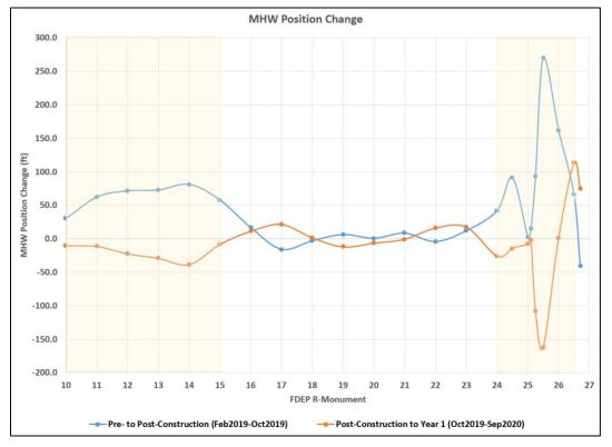
Figure 9: MHW Position Change (Highlighted areas denote fill placement areas R-10 to R-15 & R-24 to R-26.5)
