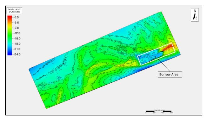
Figure 18: Post-construction Borrow Area Depths (Survey 19-247, August 2019)
