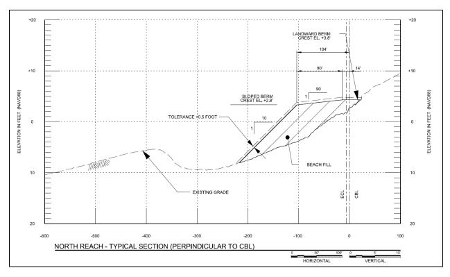
Figure 2: Typical profile and beach fill template for the federal project
