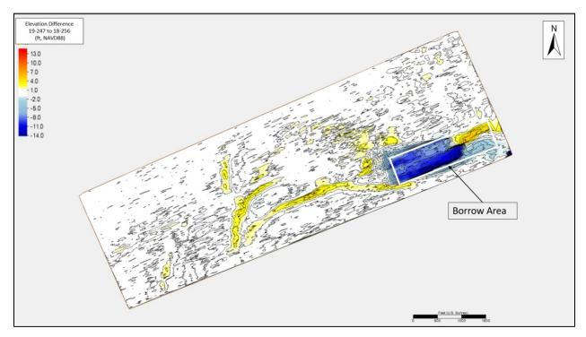
Figure 20: Borrow Area Pre To Post-Construction Bathmetry Change
