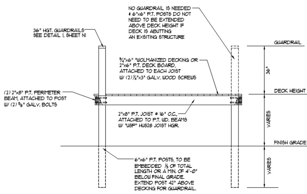
**A-A TYPICAL WOOD FRAME DECK SECTION**
