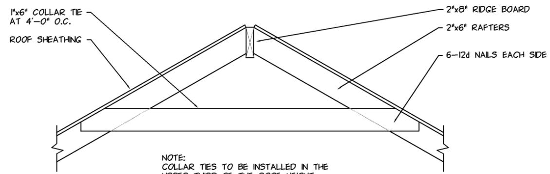
**ROOF BRACING DETAIL** (4)
