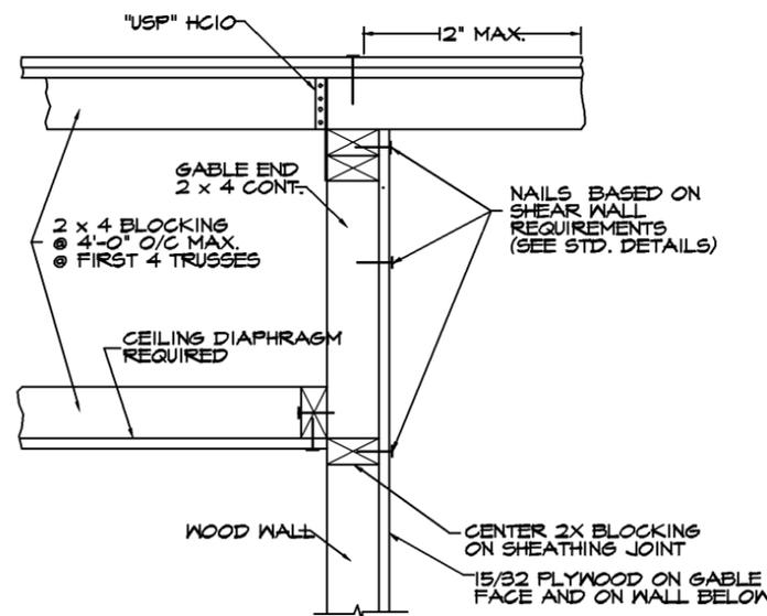
GABLE ENDWALL, BALLOON FRAMING FOR ROOF RAFTERS (10) S1 SCALE: N.T.S.
