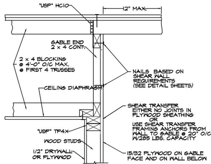
GABLE ENDWALL, PLATFORM FRAMING FOR ROOF TRUSSES (9) S1 SCALE: N.T.S.
