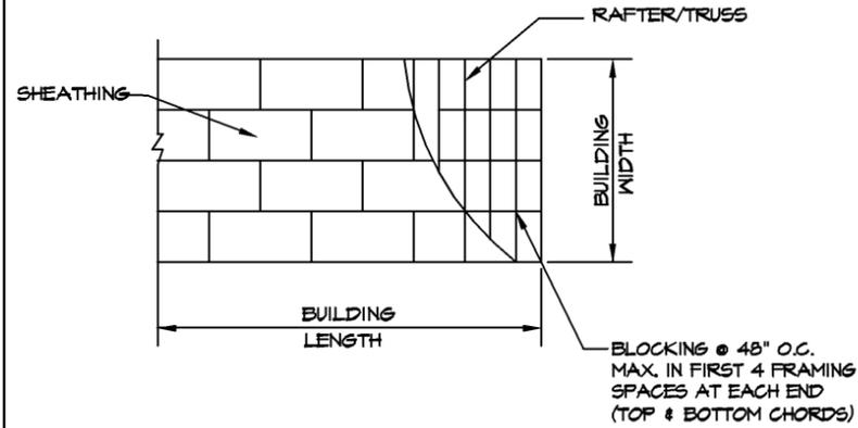
ROOF SHEATHING LAYOUT FOR GABLE ROOFS (2) S1 N.T.S.
