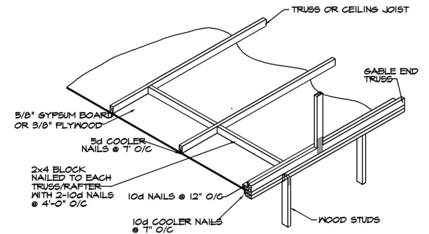
CEILING CONNECTION TO GABLE ENDWALL FOR CEILING DIAPHRAGMS (11) S1
