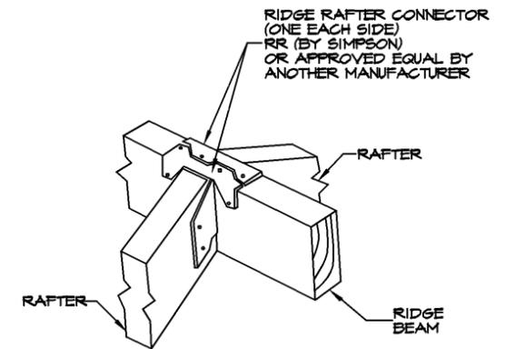
TYP. RIDGE RAFTER CONNECTOR DETAIL (8) S1 SCALE: N.T.S.
