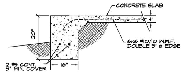
MONO. SLAB ON GRADE FOOTING FOR WD. FRAMED EXT. BRG. WALLS (1) S1 N.T.S.
