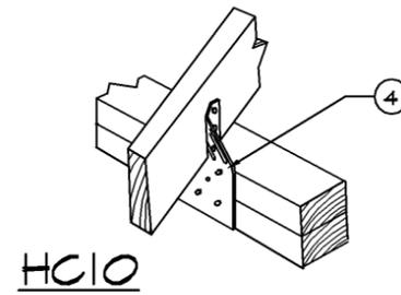
HURRICANE CLIP @ EXT. BEARING WALL (3) S1 FOR UPLIFT LOADS UP TO 1105 LBS.
