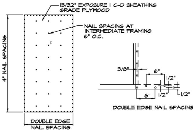
WOOD EXTERIOR WALL PANEL ATTACHMENT (5) S1 SCALE: N.T.S.
